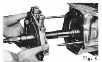
**Note:** If the rear support is stuck to the transmission case, it can be loosened by tapping lightly with a soft mallet.
