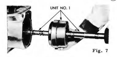
REMOVAL OF POWER UNIT #2 (SUN GEAR, REVERSE PLANET PINION CARRIER, OVERRUNNING CLUTCH AND REAR CLUTCH ASSEMBLIES)
